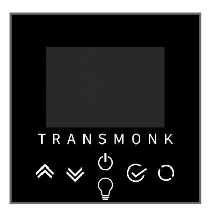
The controller is designed/programmed to auto- control speed of Motor /Actuator or Damper based on set temperature with an analog signal (0—10 VDC / 0—20 mA / PWM). The supply voltage for this controller is 230V AC 50-60Hz. The output voltage is adjusted from 0 to 10 as per feed temperature points. It is also equipped to take feedback from the equipment and display it on screen. It has user friendly button interface to set the desired temperature limits.
